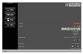
2. Under "Application Settings," set the "Default display device" to the instrument you will be using for calibration.
