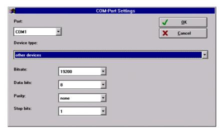
In the dialog "COM-Port Settings" you can define the serial communication port to which your measuring device is connected. In the main window you can check by the above shown pictures if a connection at the indicated interface port could be established. For device types unknow to KeyWizard you have to enter the communication parameters.
